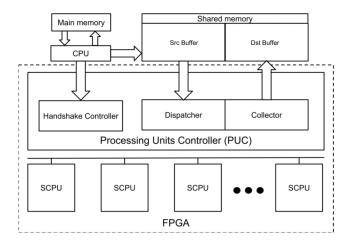
Figure 1: Collision detection accelerator system.
