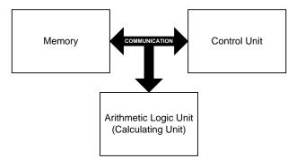
Figure 1 shows the first structure of a processor that we start with for the ORCS framework. This is similar to the basic architecture proposed by Von Neumann [11]. Basically, we take the approach where data and the program are both stored in the memory, and a controller moves information
