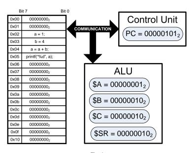
$\label{eq:Fig. 4} Fig. \ 4$  An ORCS machine with memory details and registers
