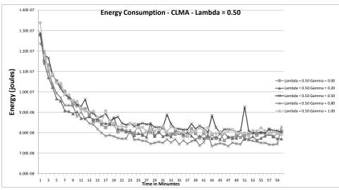
Fig. 1. Energy consumption results over 60 minutes for Lambda = 0.50 and Gamma changing
