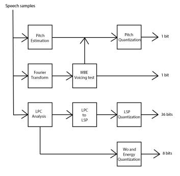
Fig. 2. Codec2 Encoder Block Diagram [2]
