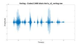
Fig. 6. Codec2 output of the hts1a.raw processed in Verilog
