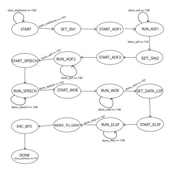
Fig. 4. FSM model of the Codec2 encoder for one FRAME (20 ms)
