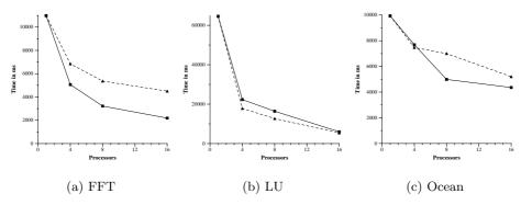
**Fig. 1.** SPLASH-2 M4 vs M4-pthread executions with 1, 4, 8 and 16processors. Solid line is the M4 executions, and dashed line is M4-pthread executions
