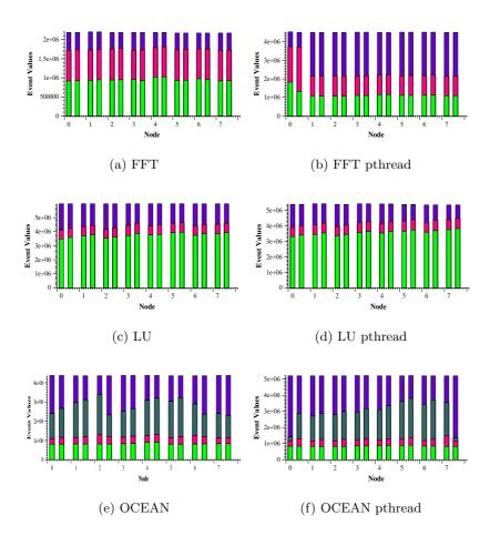
**Fig. 2.** SPLASH-2 M4 and M4-pthread execution breakdowns on 16 processors. For (a), (b), (c), and (d) the lower boxes show compute time, the middle boxes show data time, and the top boxes show barrier time. For (e) and (f) the lower boxes show compute time, the next boxes show data time, the 2nd highest boxes show lock time, and finally, the top boxes show barrier time
